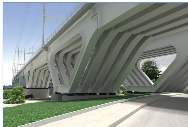
Delta Frame Pier Design
