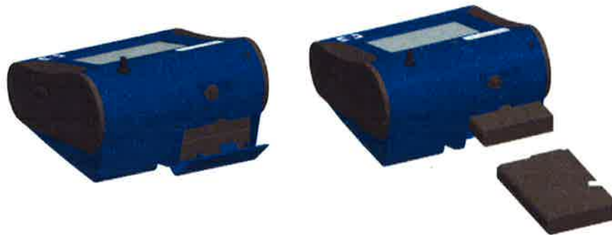
Figure 2-1: Batteries into Desktop Unit
