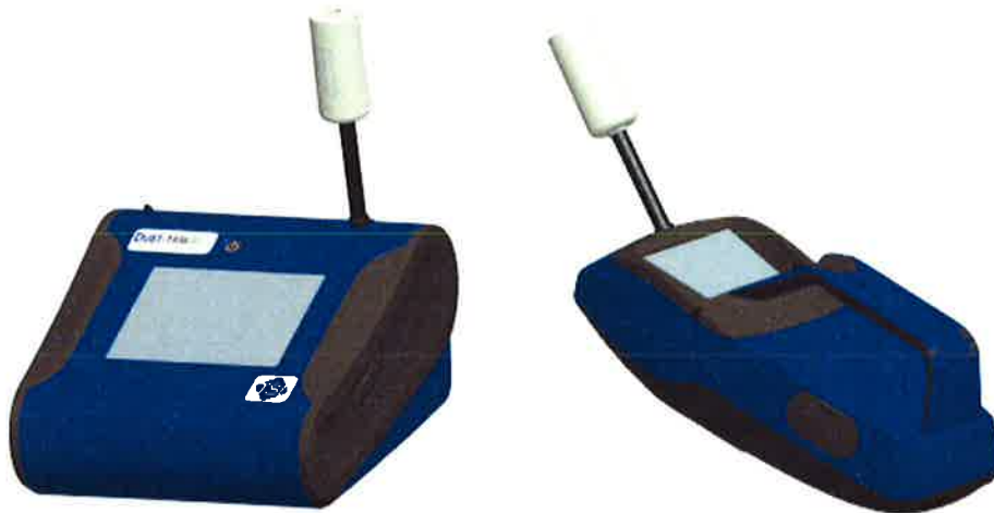
Figure 4-1: Attach Zero Filter to Inlet
