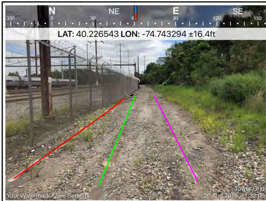
Photo 1: The photo shows the approximate location of the 5.5-foot diameter storm line along the access road, an electric line, and an unknown line. The approximate photo location, direction the photo was taken, and the date and time of the photo is presented.
