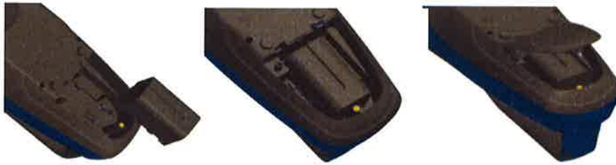
Figure 2–2: Batteries into Handheld Unit
