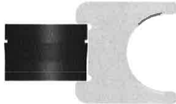
Figure 4-10: Replace Mesh in Filter Holder
