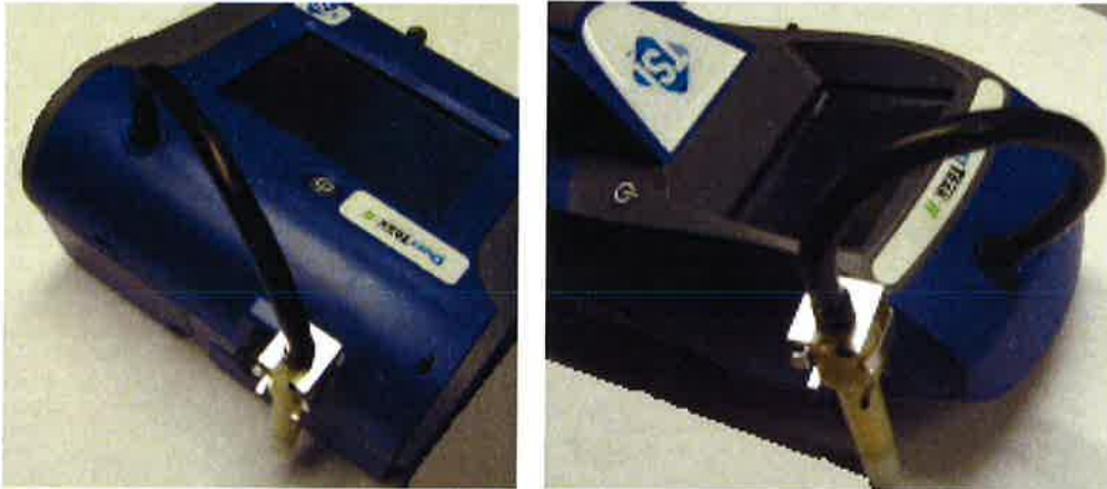
Figure 2-5: Installing Dorr-Oliver Cyclone
