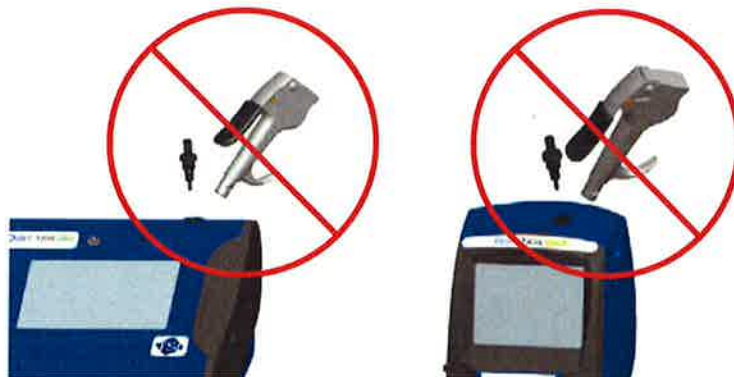
Figure 4-3: Do NOT Blow into Instrument
