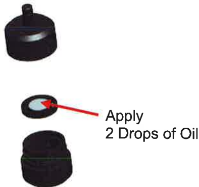
Figure 4-4: Apply 2 Drops of Oil to Impactor Plate
