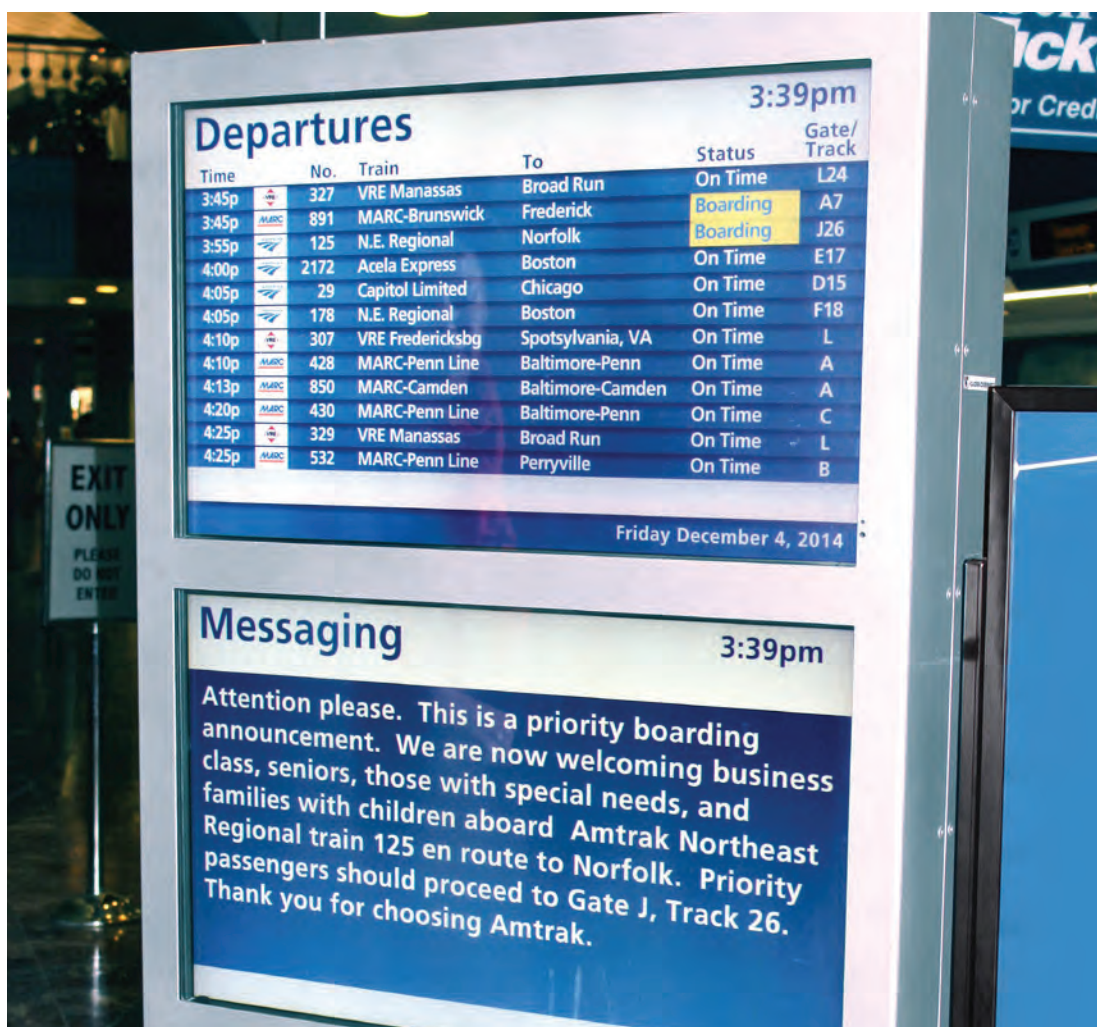
Passenger Information Display Systems (PIDS) is an integrated audio-visual messaging system that provides train information and messaging (including boarding announcements, passenger paging, general announcements and emergency messages) at both staffed and unstaffed stations.
