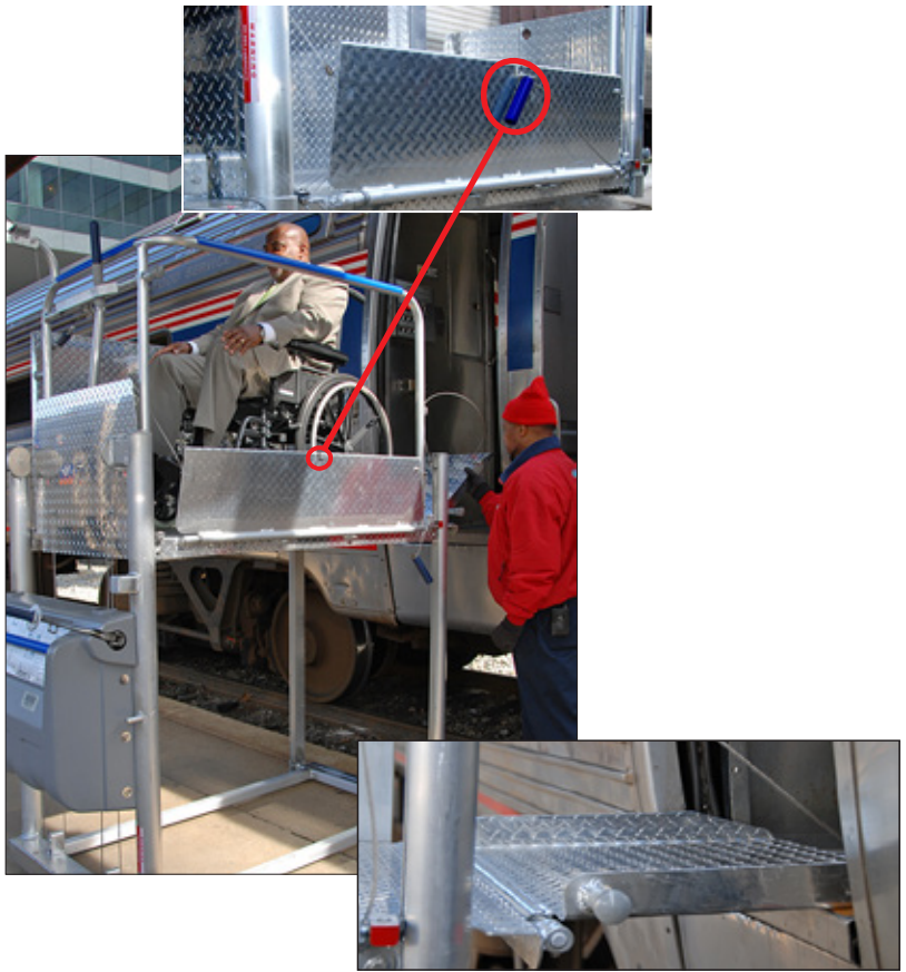
Figure 11-5 – Bridge Ramp Release Handle Figure 11-6 – Lowering Bridge Ramp Figure 11-7 – Bridge Ramp Overlapping Vestibule Floor
