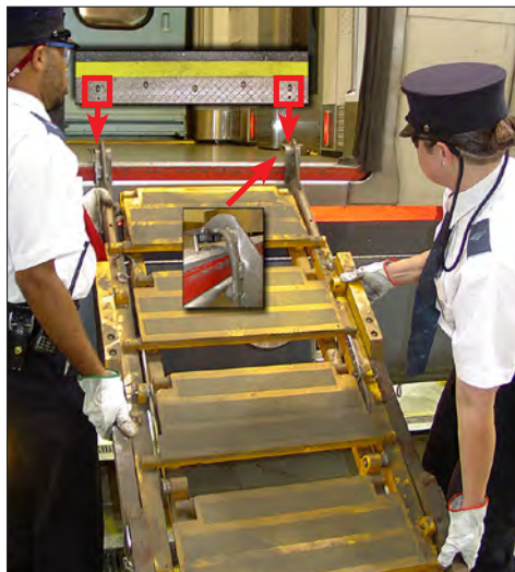
Figure 1-14 – Secure folding stairs to car body
