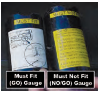
Figure 12-1 – Must Fit (GO) Gauge and Must Not Fit (No/Go) Gauge
