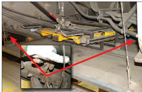
Figure 1-12 – Lower storage compartment latches and safety cables
