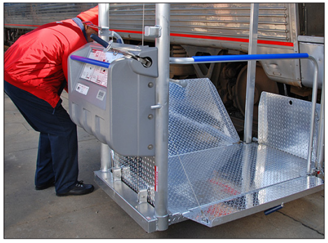
Figure 11-3 – Lowering Ground Ramp
