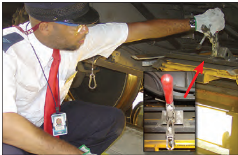
Figure 1-13 – Release folding stairs hold-down clamp
