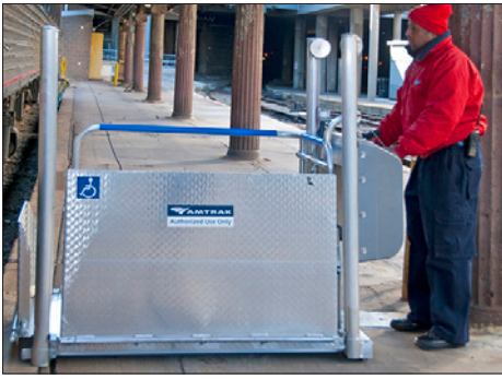
Figure 11-2 – Positioning Lift Next to Train
