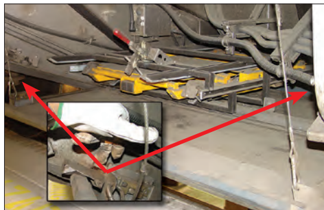
Figure 1-12 – Lower storage compartment latches and safety cables
