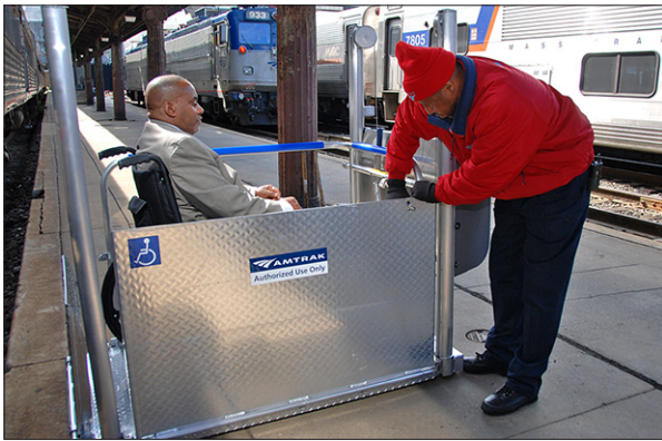
Figure 11-4 – Closing Ground Ramp
