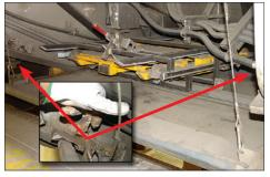
Figure 1-12 – Lower storage compartment latches and safety cables
