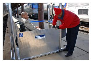
Figure 11-4 – Closing Ground Ramp
