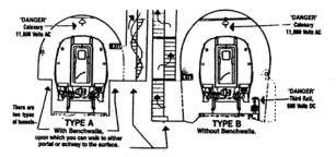
Figure 1-16 - Tunnel Hazards
