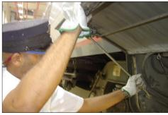
Figure 1-11 - Secure the door safety bar
