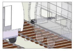
Figure 1-4 – Turn transfer bridge  $90^\circ$  and carefully unfold top section (one fold) as shown.
