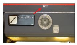
Figure 1-10 – Upper storage compartment door, latch and decal
