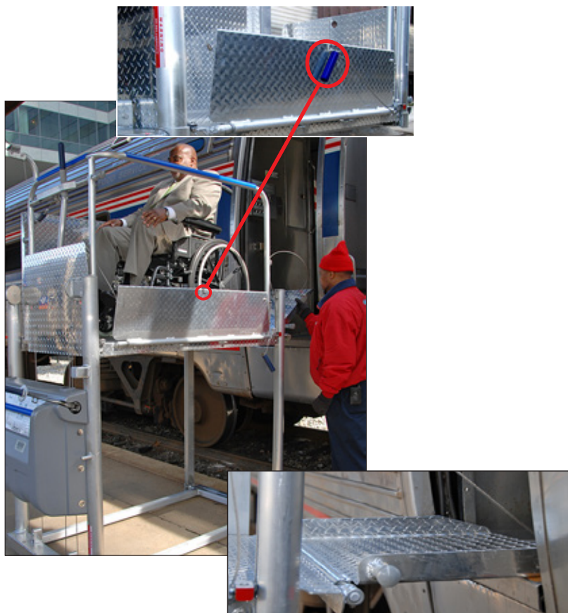
Figure 11-5 – Bridge Ramp Release Handle Figure 11-6 – Lowering Bridge Ramp Figure 11-7 – Bridge Ramp Overlapping Vestibule Floor
