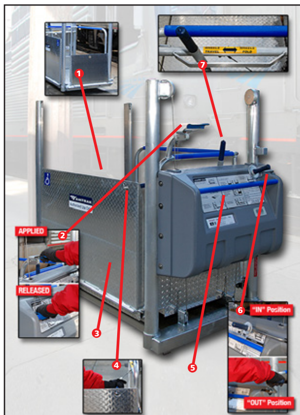
Figure 11-1 – Wheelchair Lift Components
