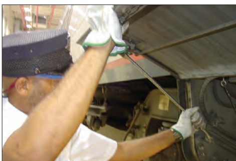
Figure 1-11 – Secure the door safety bar
