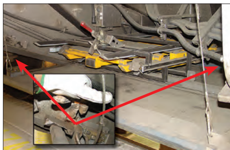
Figure 1-12 – Lower storage compartment latches and safety cables
