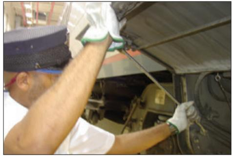
Figure 1-11 – Secure the door safety bar
