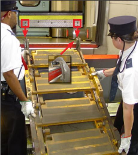
Figure 1-14 – Secure folding stairs to car body
