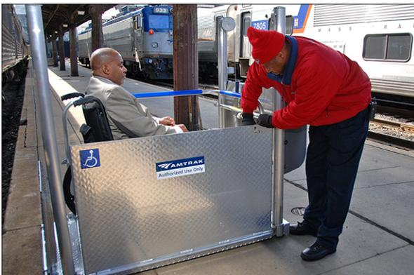
Figure 11-4 – Closing Ground Ramp
