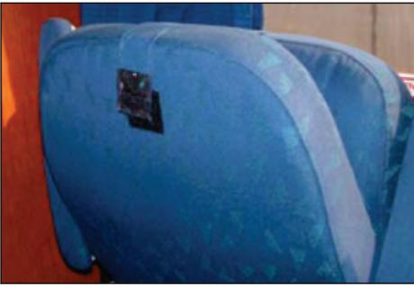
Figure 12-7 – Velcro Fabric Strap Securing Seat Cushion in Folded Position
