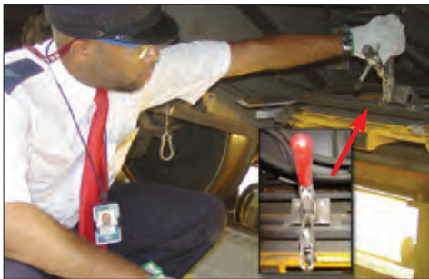
Figure 1-13 – Release folding stairs hold-down clamp
