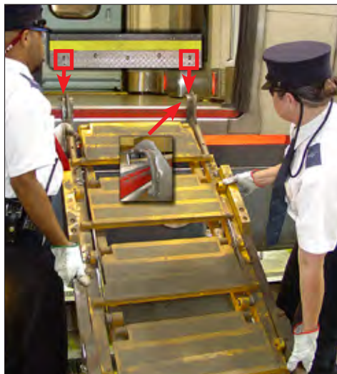
Figure 1-14 – Secure folding stairs to car body
