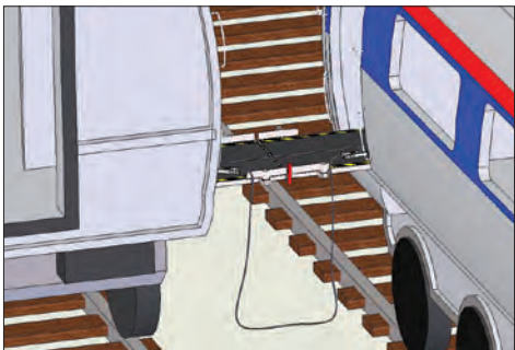
Figure 1-8 – Unfold transfer bridge to flat position and insert Safety Lock Bar with red handle up.
