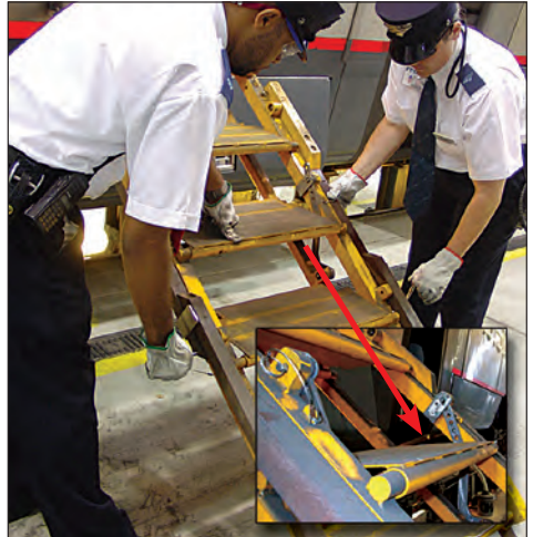
Figure 1-15 – Level stair steps
