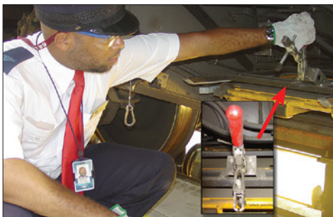
Figure 1-13 – Release folding stairs hold-down clamp
