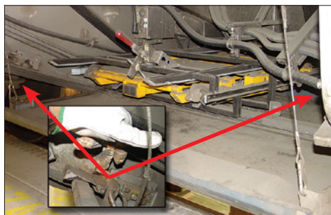
Figure 1-12 – Lower storage compartment latches and safety cables
