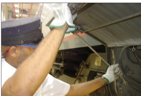
Figure 1-11 – Secure the door safety bar
