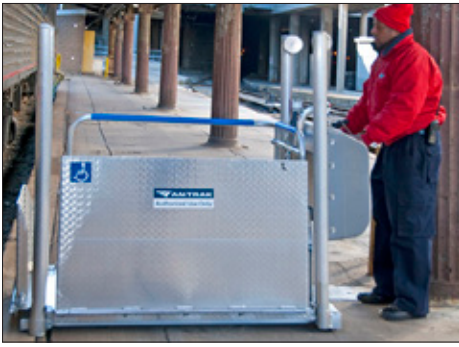
Figure 11-2 – Positioning Lift Next to Train
