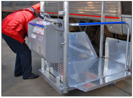
Figure 11-3 – Lowering Ground Ramp
