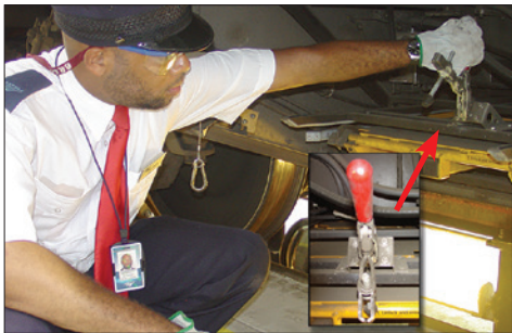
Figure 1-13 – Release folding stairs hold-down clamp
