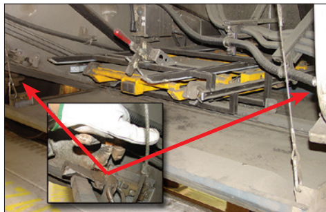
Figure 1-12 – Lower storage compartment latches and safety cables
