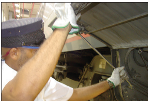
Figure 1-11 – Secure the door safety bar
