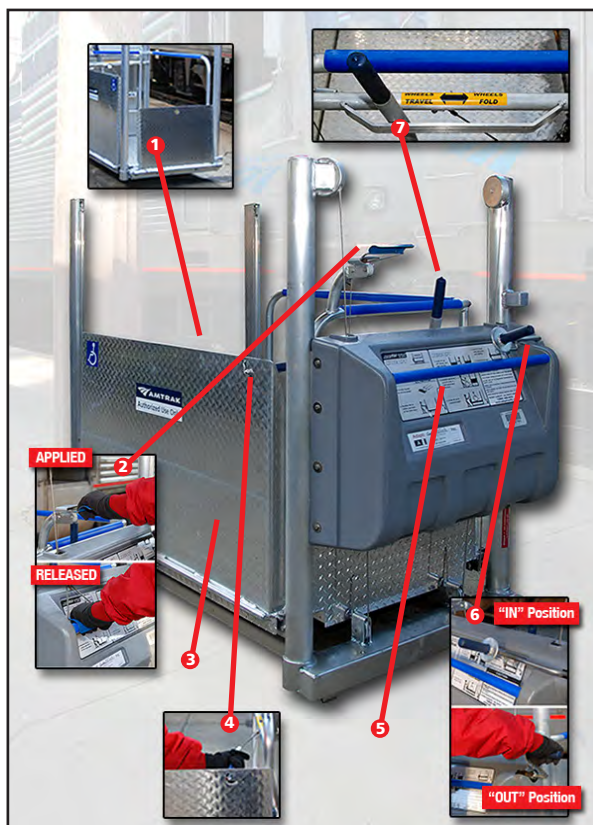
Figure 11-1 – Wheelchair Lift Components
