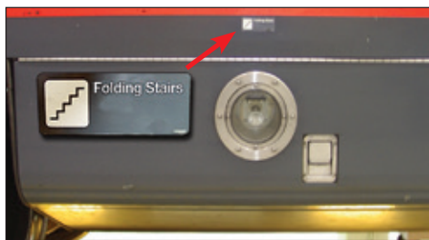
Figure 1-10 – Upper storage compartment door, latch and decal
