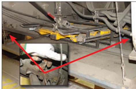
Figure 1-12 – Lower storage compartment latches and safety cables
