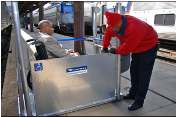
Figure 11-4 – Closing Ground Ramp
