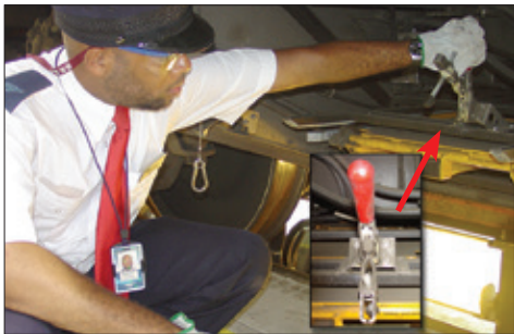
Figure 1-13 – Release folding stairs hold-down clamp
