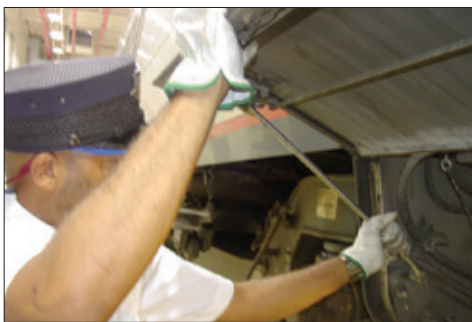
Figure 1-11 – Secure the door safety bar
