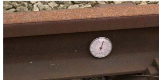
Figure 4 Placement of Rail Thermometer
