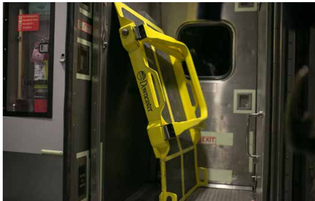
At left: ADA Platform bridge plate on the Downeaster, 145-mile regional passenger train service managed by the Northern New England Passenger Rail Authority and operated by Amtrak.
