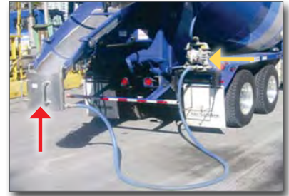
Figure 8. Chute washout bucket and pump
