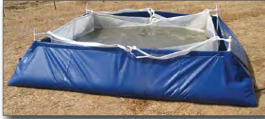
Figure 11. Vinyl washout pit with filter bag
