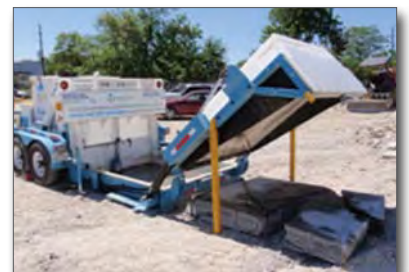
Figure 17. Delivering hardened concrete to a recycler
