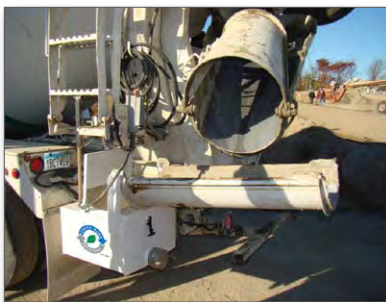
Figure 7. Chute washout box
