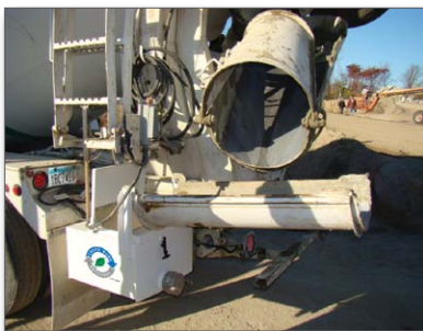
Figure 7. Chute washout box
