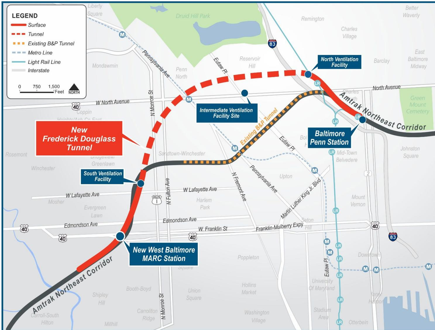
The Selected Alternative would require three ventilation facilities to ensure proper ventilation of the proposed tunnels: a North Ventilation Facility located near the north portal; a South Ventilation Facility near the south portal; and an Intermediate Ventilation Facility (IVF) between the north and south portals located at street level, connected to the tunnel bores by a vertical shaft and connecting tunnel.
