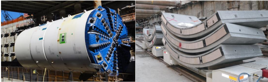
Figure IV-31: Tunnel Boring Machine and Precast Concrete Segments
