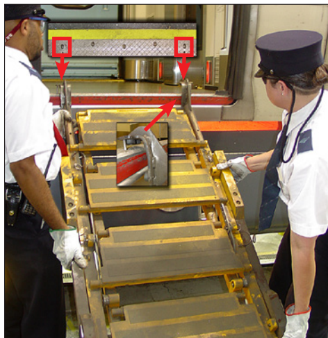
Figure 1-14 – Secure folding stairs to car body
