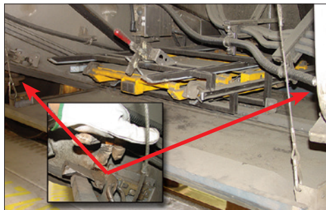
Figure 1-12 – Lower storage compartment latches and safety cables
