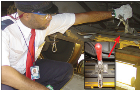
Figure 1-13 – Release folding stairs hold-down clamp
